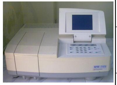
Used For quantitative identification of the elements of solid or liquid samples as well as anions like NO<sub>2</sub>, NO<sub>3</sub> etc
