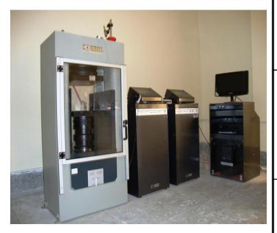
Used For the determination of uni-axial and triaxial strength, modules of elasticity, strength index of hard rocks
