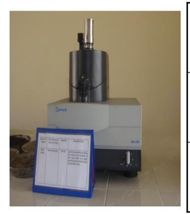
**Used For:** grinding hard rock of two R&D projects of IMMM has been carried out.
