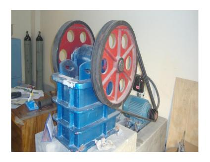
**Used For:** grinding hard rock samples of R&D projects.
