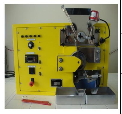
**Used For:** The mineral separation from river sand and grinded hard rock of three R&D projects of IMMM has been carried out.
