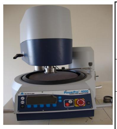
**Used For:** The thin section slide of rock and minerals for petrological sample analysis by polarizing microscope is prepared by this unit. The petrological slide for 4 students of Rajshai university for their academic research have been prepared.
