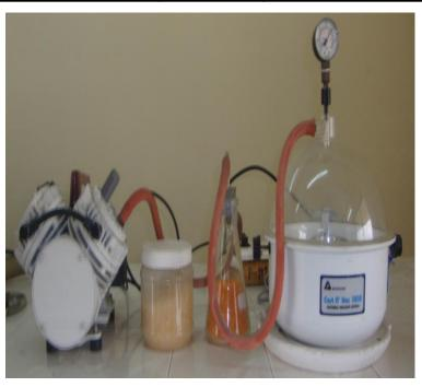
**Used For:** The thin section slide of rock and minerals for petrological sample analysis by polarizing microscope is prepared by this unit.
